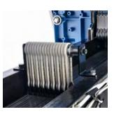
SMIT GS980 shedding motion, optimized in combination with the latest dobby models, ensures minimal vibrations of heald frames, with increased warp efficiency at top speed.
