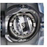
The Rapier Drive, carried out by a "spherical crankshaft" and one gear stage, ensures minimum weft cutting, transfer and release speed, with the highest regularity in weft insertion.
